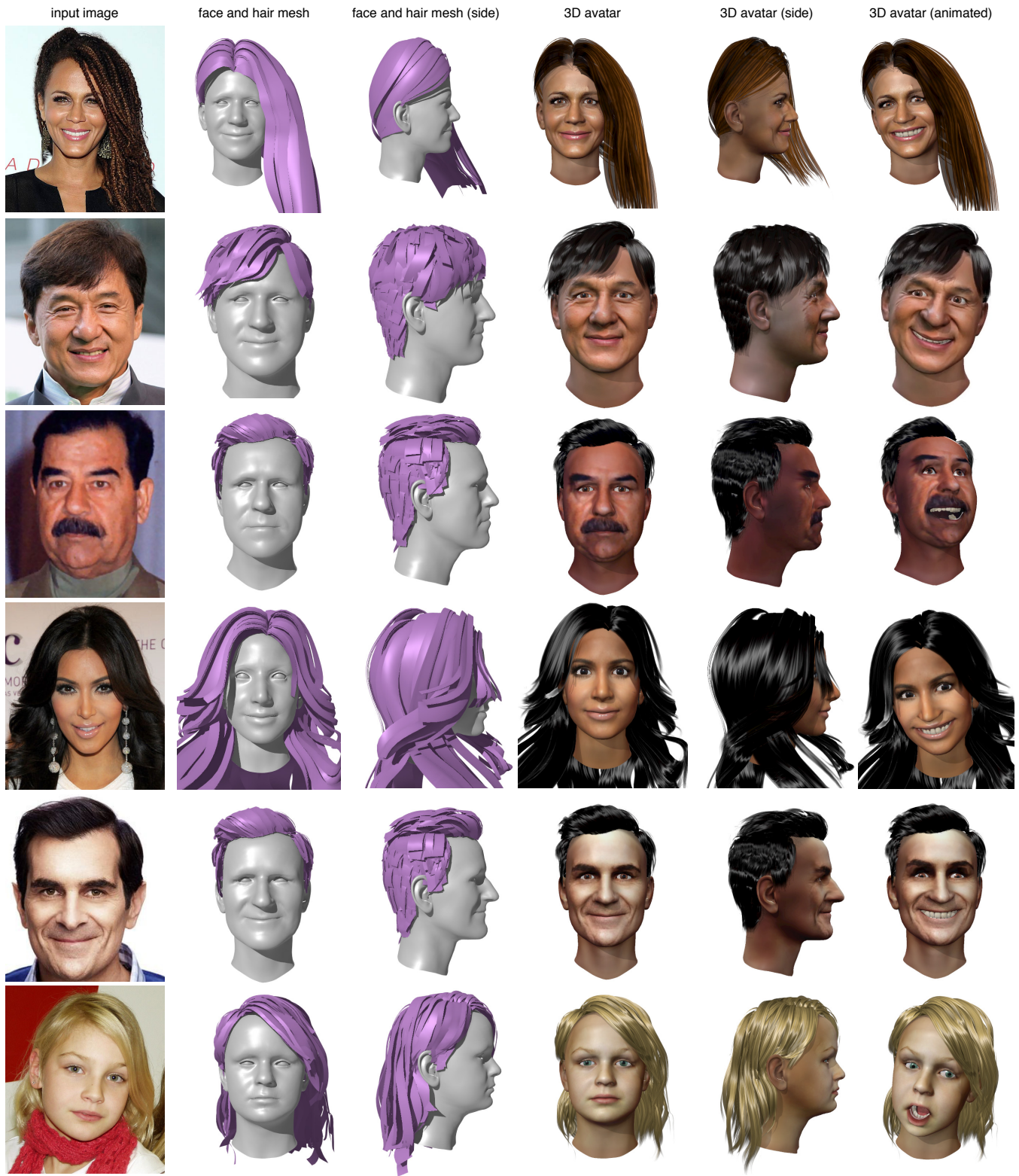
Fig. 10. Our proposed framework successfully generates high-quality and fully rigged avatars from a single input image in the wild. We demonstrate the effectiveness on a wide range of subjects with different hairstyles. We visualize the face meshes and hair polystrips, as well as their textured renderings. Original images courtesy of Getty Images.
